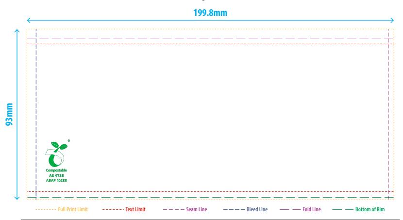
NOTE: Ensure that any objects or images that extend beyond the Full Print Limit are <u>cropped</u> (not clipped) for the curving to work correctly.
